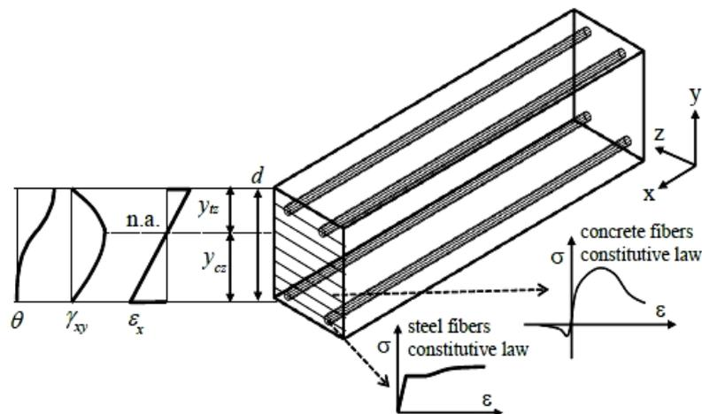
Fig. 1 – Fiber Element Scheme – definitions [5], [6].
