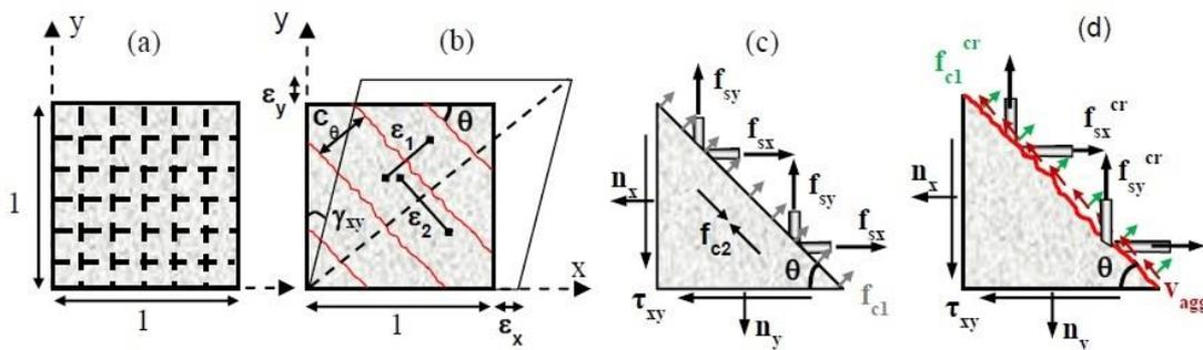
Fig. 2 – a) RC smeared-cracking membrane element, b) average strains ( $C_\theta$ : spacing of cracks inclined at  $\theta$ ) c) average stresses and d) local stresses [5], [6].
