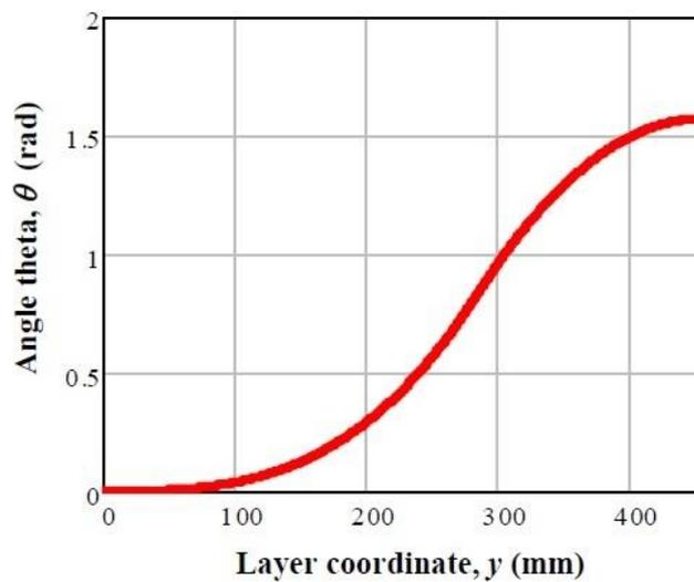
Fig. 4 – Shape function for angle theta ( $\theta$ ) of inclination of principal stresses/strains [5], [6].
