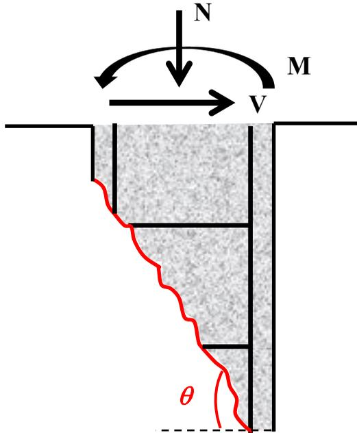
Figure 2-3: Angle inclination of the primary shear crack.
