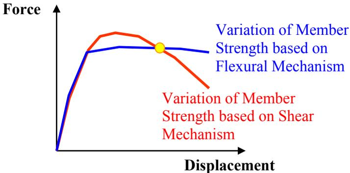
Fig. 2-1: Capacity curve due to flexural or shear mechanism.
