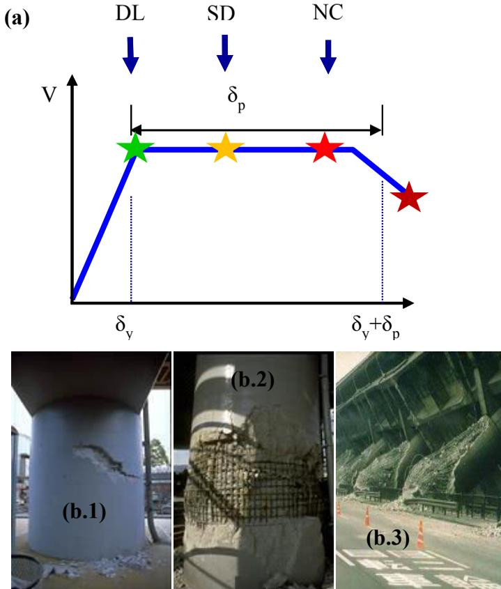
Fig.2-2: Damage of bridge columns: a) Member resistance curve and definition of limit states according with EN 1998-3 (2005).
