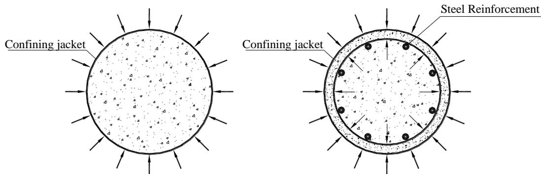
**Fig. 1** Circular Concrete Section confined by steel stirrups and/or FRP Jackets.
