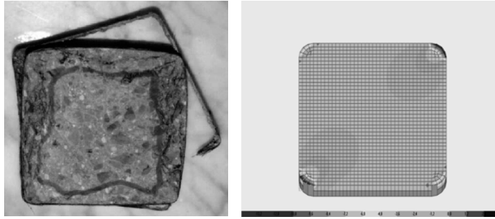
Figure 1. Cross-section of a square column: left, test (from Campione and Miraglia 2003); right, FEM model.
